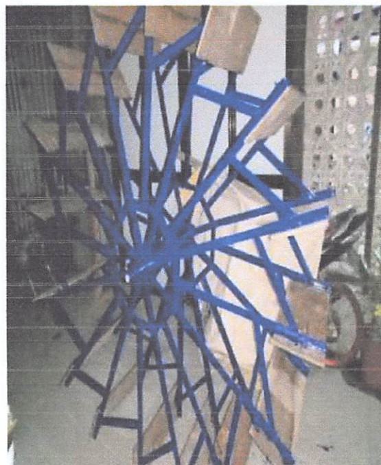
Figure 9. Waterwheel pico-hydropower plant
