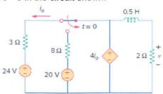
5. The switch in the figure below has been in position a for a long time. At t = 0, it moves to position b. Calculate i(t) for all t > 0.
