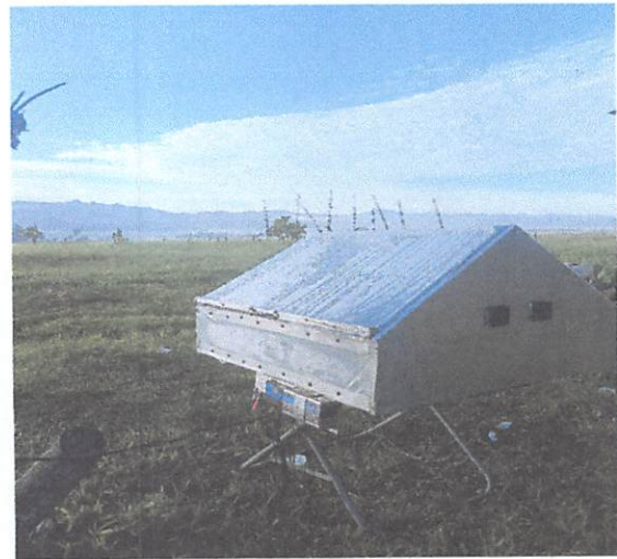
Figure 13. Automated solar powered chamber
