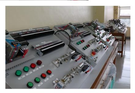
Pneumatic and Electro – Pneumatic with PLC Training System
